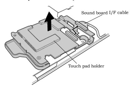
Figure 4-24 Removing the touch pad holder
